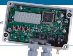
The FlowGuard 6279 is an advanced processor transmitter aimed for the standard pressure measurement tasks. It's designed with the user and installer in mind. The 6279 eliminate many of the problems that traditional sensors suffer from and provide as much flexibility as possible.
